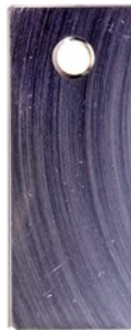
Figure 5.4 Appearance of 1.4404 coupon after 6 months of exposure in the artificial SBY geothermal brine at 100 °C
