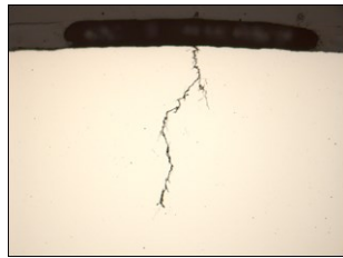
Figure 2.7 Stress corrosion cracking
