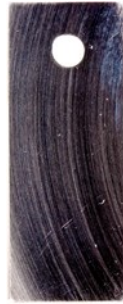
Figure 6.4 Appearance of 1.4562 coupon after 6 months of exposure in the artificial SBY geothermal brine at 100 °C
