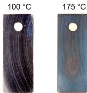
Figure 6.10 Appearance of 1.4562 coupons after 6 months of exposure in the artificial SBY geothermal brine at 100 °C and 175 °C, respectively
