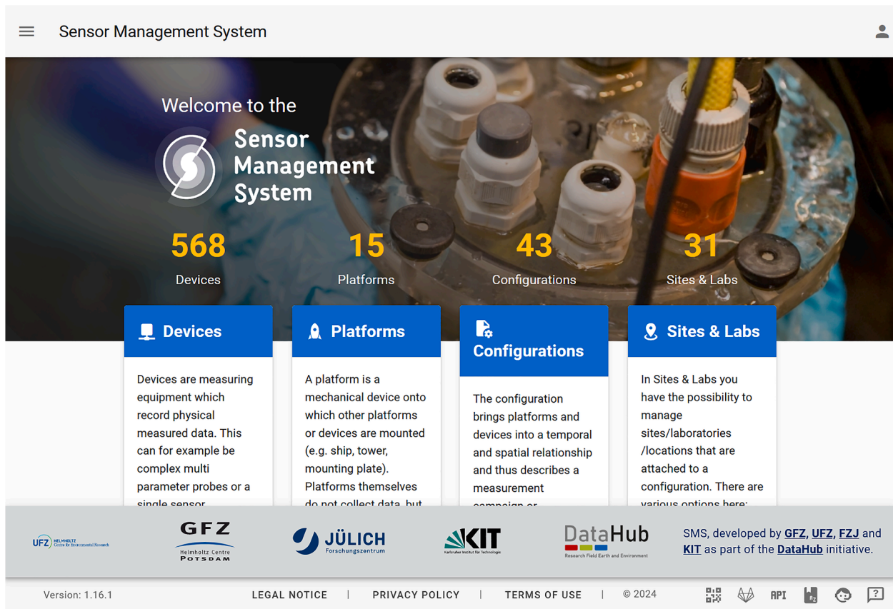
Fig. 2. Front-End SMS. The sensor management system (SMS) is designed to handle the acquisition and management of metadata from various sensors.
