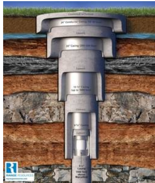
Fig. 1: Sketch of a sequence of cemented casing pipes from a typical wellbore (not to scale).
