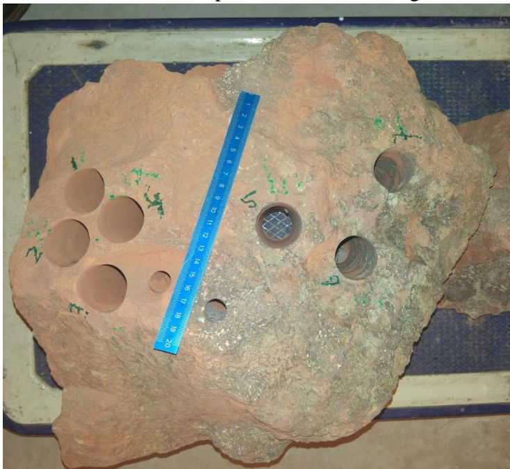
Figure 1, example of the provided a provided sample block (this case: VIB8_IC_01), with locations of the drilled cores indicated on the block. Note the ruler for scale.
