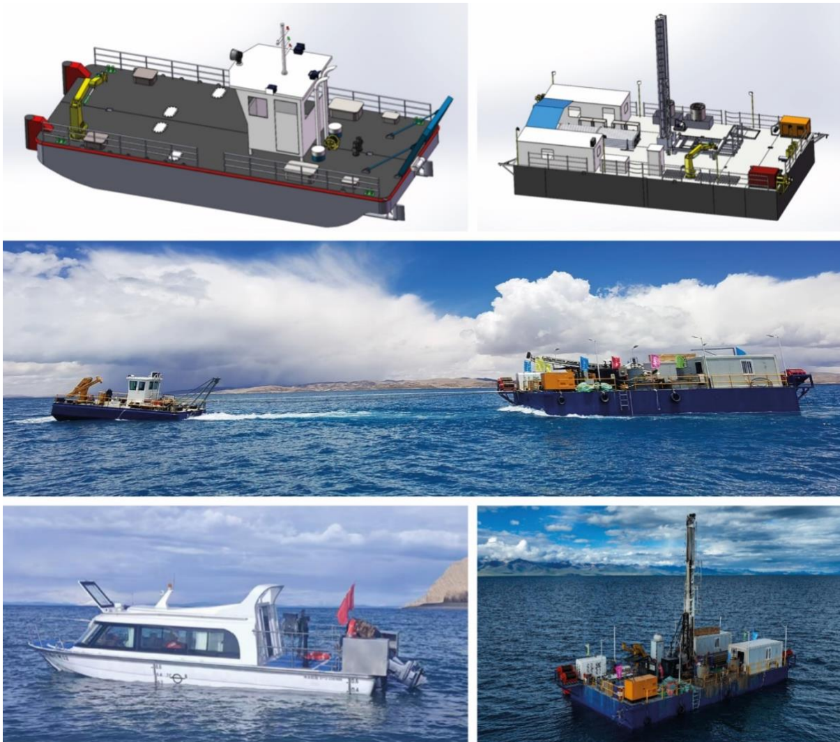
Fig. 7: Technical drawing of the tugboat (top left) and the barge (top right) built for the NamCore project. The tugboat was used to tug the barge to the drill site (centre). Transfer between the campsite and barge at drill site (bottom right) was carried out with the transfer boat (bottom left).
