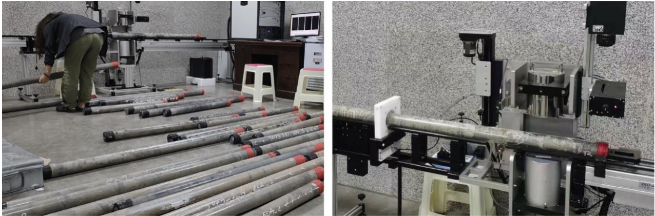
Fig. 11: MSCL core scanning at the Institute of Tibetan Plateau Research, Chinese Academy of Sciences, Lhasa Campus.
