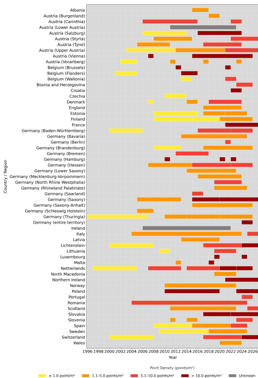
Figure 3. Years of acquisition of airborne laser scanning campaigns conducted by governmental institutions in Europe, including point density information where available. Note that the information provided is likely incomplete, both in terms of available data and their metadata, as these are documented to varying degrees and reliability. In addition, the years of acquisition may also include the preparation and processing time (i.e., \pm 1 year), as it is often difficult to distinguish whether only the acquisition years are reported or if they also include data processing. Similarly, it is difficult to distinguish whether point or pulse density is reported, and whether these are nominal/minimal densities or realized densities (which are often higher). Therefore, we use the single term point density.
